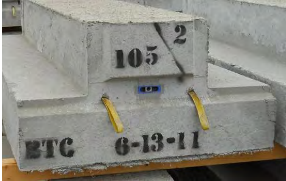
Lifting Sling Straps at Top of T Panel
